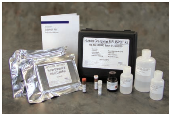
Figure 1. BD ELISPOT Human Granzyme B Kit. The kit components include two pre-coated plates and all necessary reagents: Antibody-coated Plates, Detection Antibody, Avidin-HRP, AEC Substrate/Chromogen, Assay Diluent, PBS Concentrate and Wash Concentrate.
